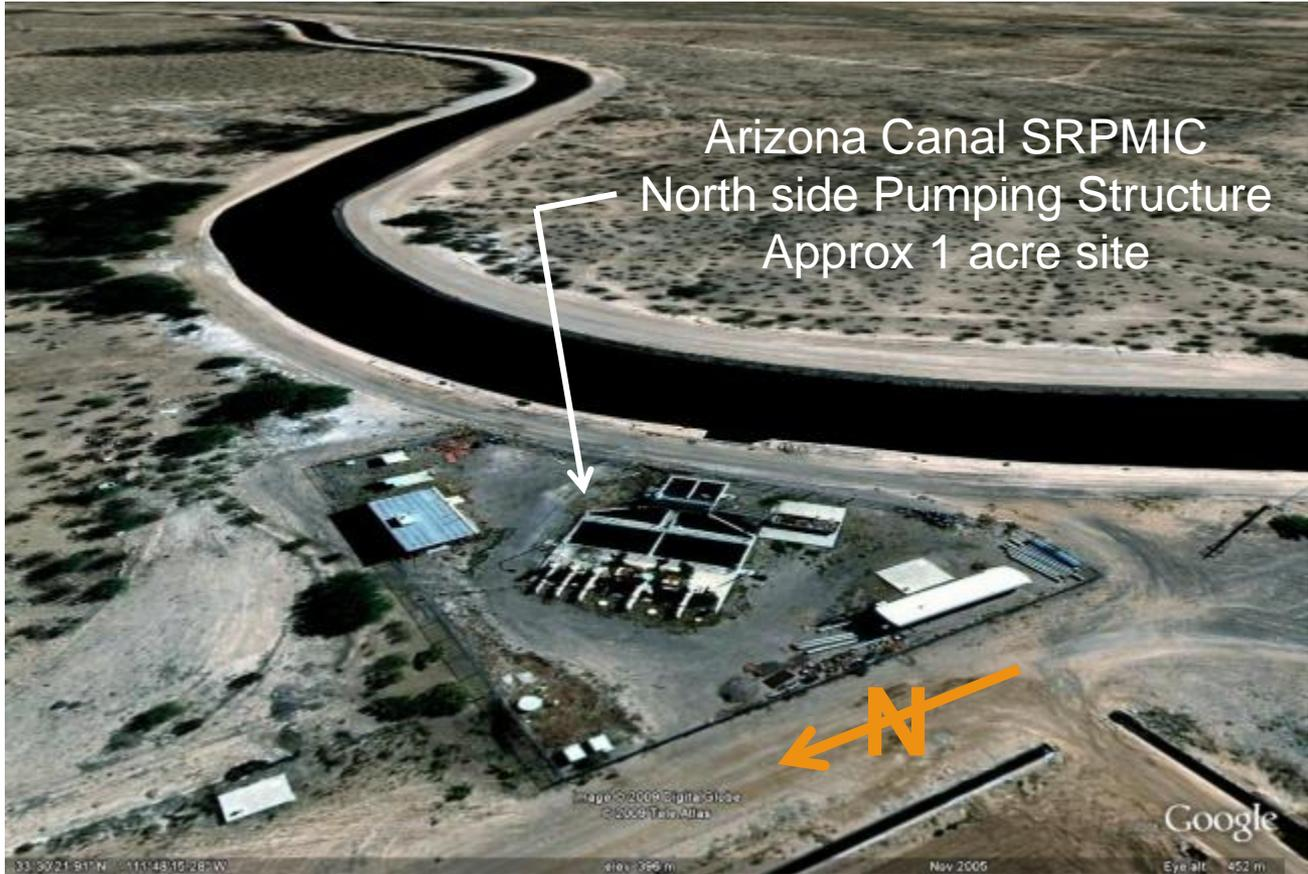
**Pump station with 5 sump pumps deliver water north about 3 miles**
