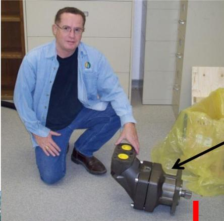
Pictured is a 335 HP hydraulic motor that replaces the electric motor
