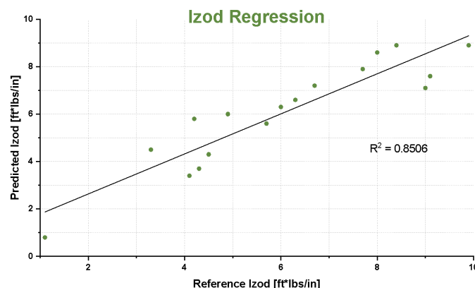
Fig. 4 shows a regression model developed for the prediction of Izod by lab IMR (MagStation II) for pellets. Its root mean square in this example is 0.85.
