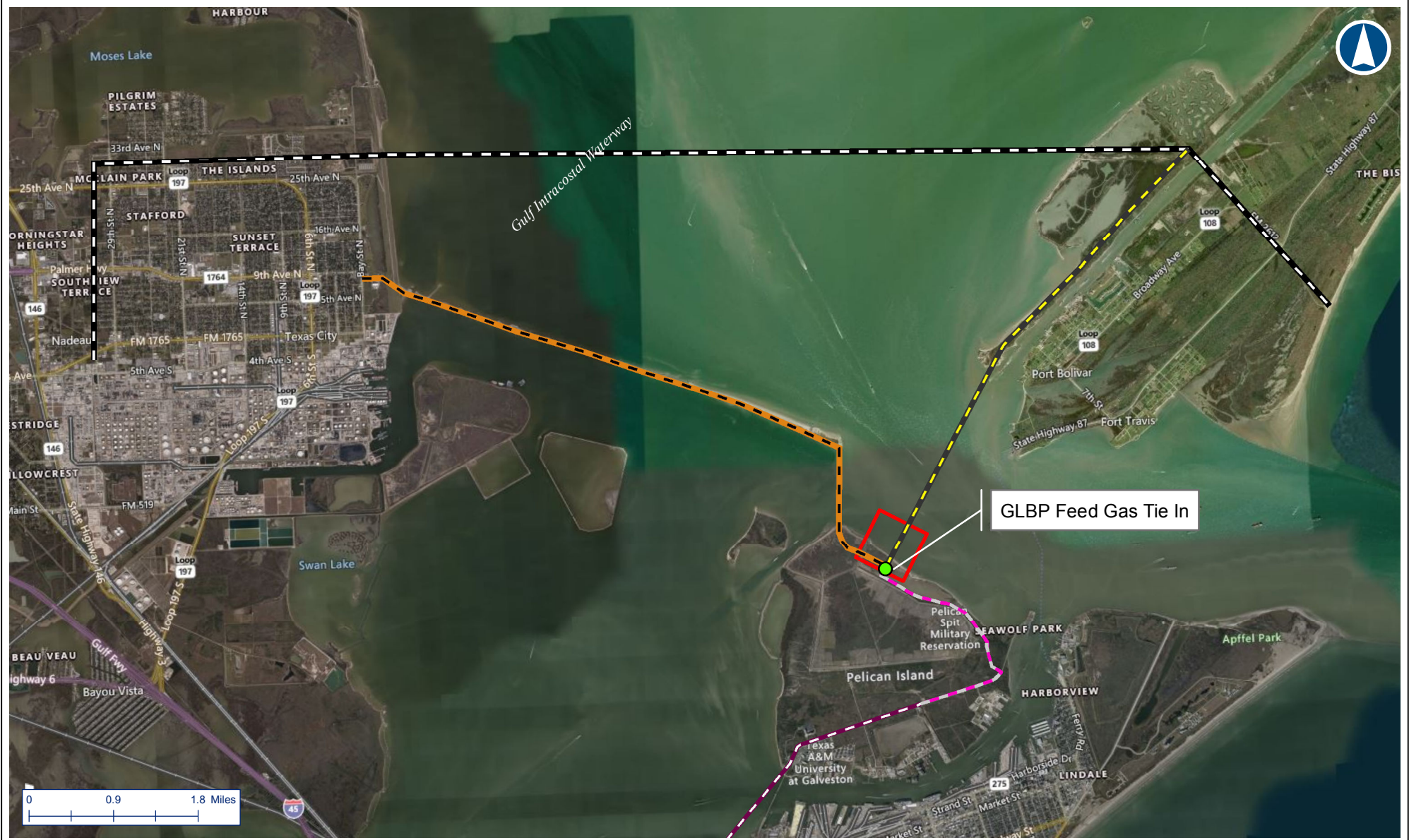
FIGURE 1-9: FEED GAS PIPELINE ALTERNATIVES - GALVESTON LNG BUNKER PORT
