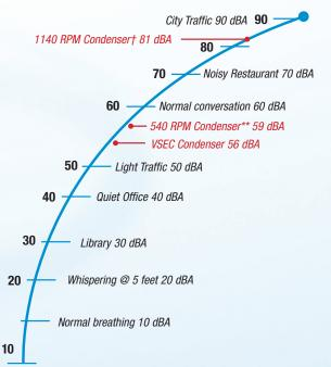
Source: Noise Pollution Clearinghouse, 2005 \* 10 Fan with EC motors \*\*12 Fan with 540 motors † 10 Fan with 1140 motors
