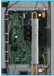
**1 Daikin Inside variable-speed compressor** – Provides up to 21 SEER cooling performance for lower energy bills compared to lower SEER, single-stage compressors.
