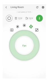
Select Fan mode only when cooling or heating is not necessary
