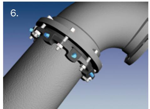
6. If removal is necessary, utilize the 5/8 inch hex heads provided. If reassembly is required, assemble the joint in the same manner as above, by tightening the wedge bolts to 90 ft-lbs. If the series 1100 restraint is removed from the pipe, be sure that all the collar bolts and wedges are in place before the restraint is reassembled.
