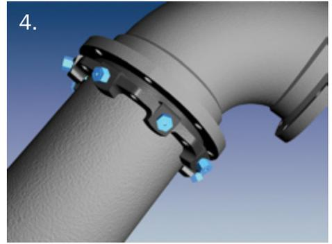
4.\* Push the gland toward the socket and center it around the pipe with the gland lip against the gasket. Insert bolts and hand tighten nuts. Make deflection after joint assembly but before tightening bolts.
