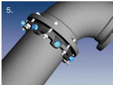
5. In large sizes (30-48 inch), five or more repetitions may be required. The use of a torque-indicating wrench will facilitate this procedure.
