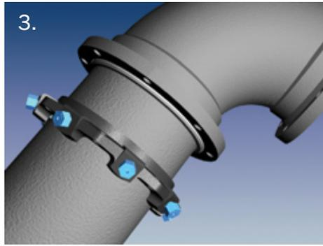
3.\* Insert the pipe into the socket and press the gasket firmly and evenly into the gasket recess. Keep the joint straight during assembly.
