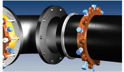
3. Lubricate and place the EBAA-Seal™ Gasket on the clean pipe following the restraint ring. (USE A TRANSITION GASKET IN PLACE OF THE EBAA-SEAL GASKET FOR STEEL AND IPS. O.D. PVC PIPE.)
