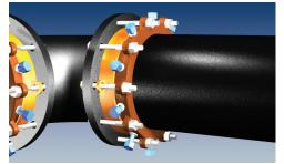
7. Tighten the actuating screws in an alternating manner until all wedges touch the pipe. Continue tightening the nuts in an alternating pattern until all the torque-limiting nuts have been twisted off.
