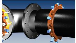
2. Cut the pipe to the required length. Clean the end of the pipe for a length approximately one foot using a wire brush if needed, removing all excess paint and foreign material. Also clean the opposing flange to be connected to the 2100. Place the 2100 restraint ring on the clean pipe with the lip facing the plain end.
