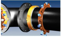
4. Place the O-ring into the groove of the 2100 Gasket Ring. (This step may have been completed at the factory, check Gasket Ring to see if O-ring is already in place.) Place the Gasket Ring on the pipe with the O-ring facing the pipe end and the gasket recess facing the EBAA-Seal (or transition) Gasket and restraint ring.
