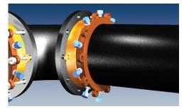
5. Bring the pipe and flanges together within the maximum assembled deflection and maximum allowable gap "L" to the flange face. Slide the gasket ring, gasket and restraint ring until contact is made with the opposing flange.
