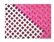
High mesh counts with high tension are a necessary part of multi-colour prints and allowing for a little
