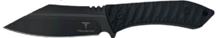
(T18) TKF318 ~ 228mm Overall 113mm 3cr12 Sheep's foot Blade 3.82mm Thick Full Tang, Black FRN Handle
