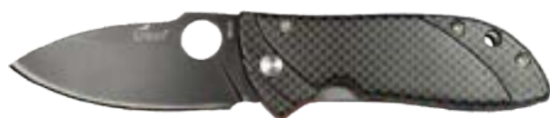
(E14) M020FB ~ 91mm Closed Imitation Carbon Fibre Handle 67mm 8cr13mov Steel Blade Thumb Hole, Lanyard Hole HRC: 55-60 Liner Lock, w/Clip
