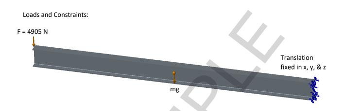
Moment of inertia,  $I_{x_r}$  von Mises stress,  $\sigma_{vm}$ , and displacement,  $\delta$ , calculations:
