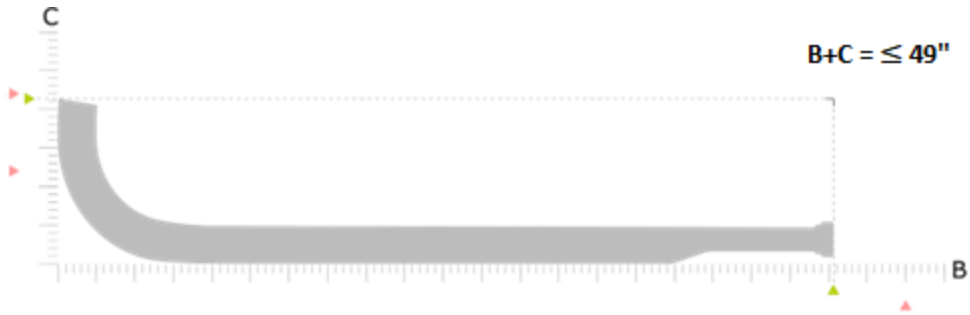
Design 4 - Illustration of a traditional goalkeeper stick within the limits of the box rule.
