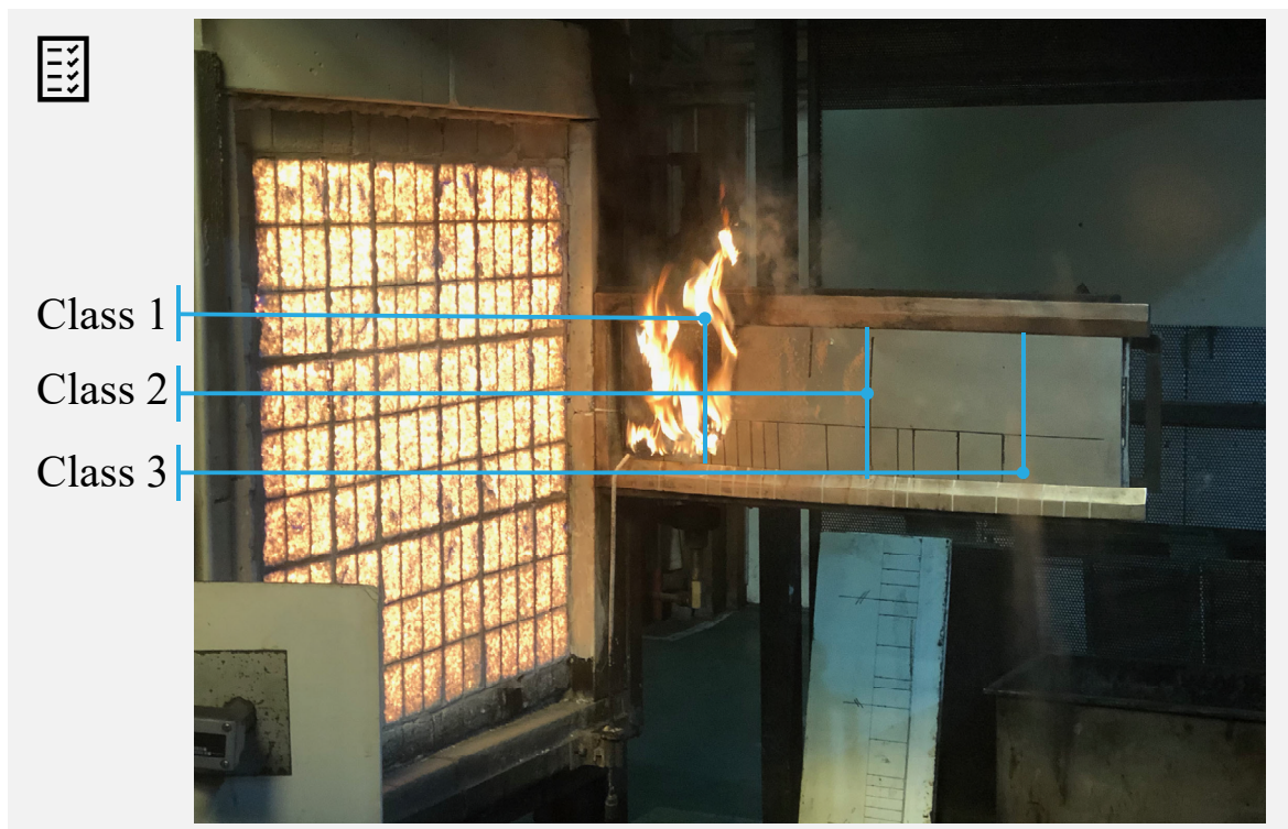
Figure 5.2: Image of BS 476-7 test in operation
