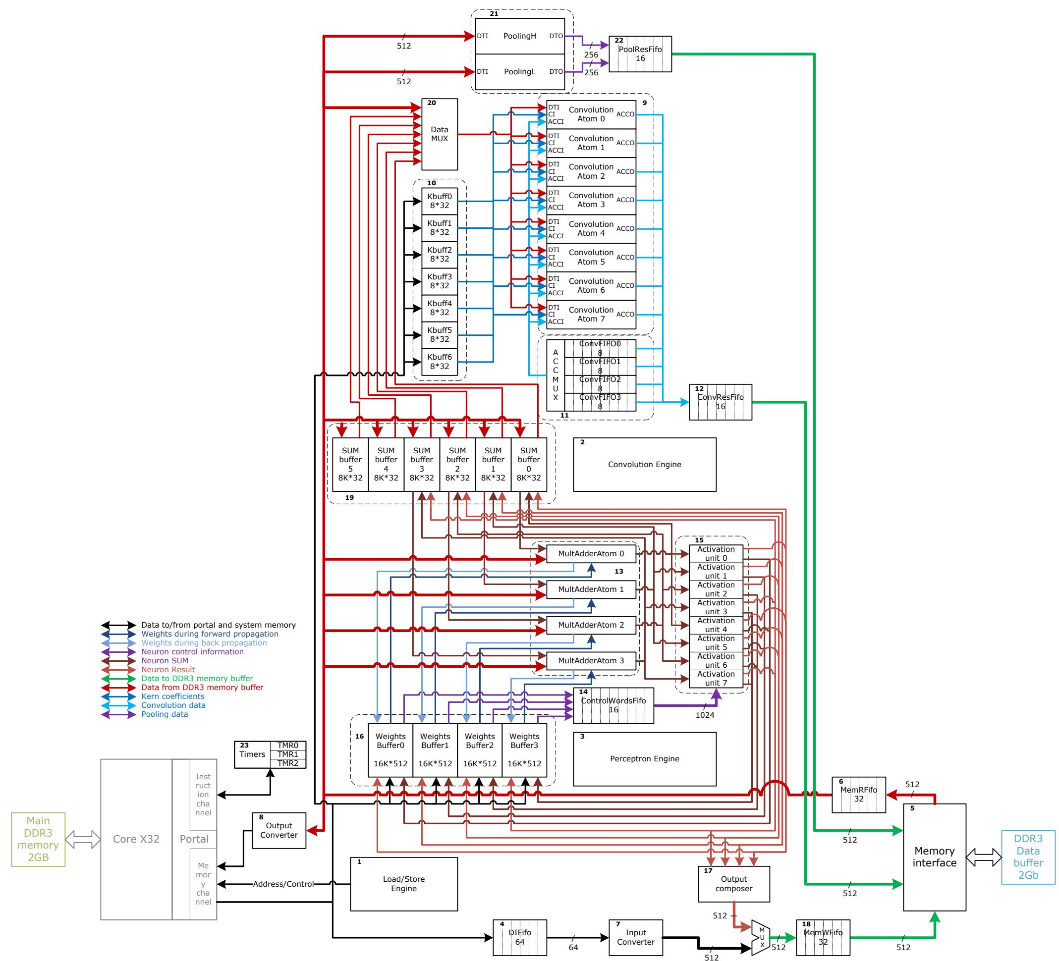
1. Load/Store engine. The engine performs NULD, NUSD, NULP, NUSP operations and loading of error values in the perceptron backpropagation instruction - NUBP.
