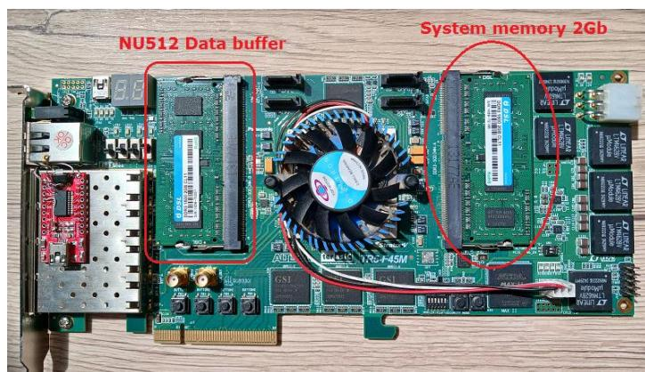
One of the channels was used as the system memory of the X32Carrier core. The second channel was used as data memory for the NU512 block. DDR3 SDRAM Controller with UniPHY v16.1 was used to connect to the memory. Its Avalon-MM interface was configured for Quarter rate mode and 512-bit bus width, operating at 150 MHz. The 5SGXEA7N2F45C2 crystal resources were used at 95%.
