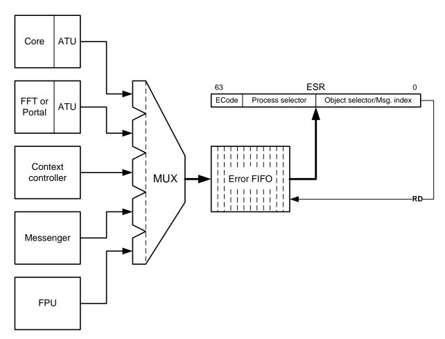
The output of the error queue is the system register ESR, which is read-only. The presence of a real value at the output queue can be determined from the non-zero state of the Error Code field.
