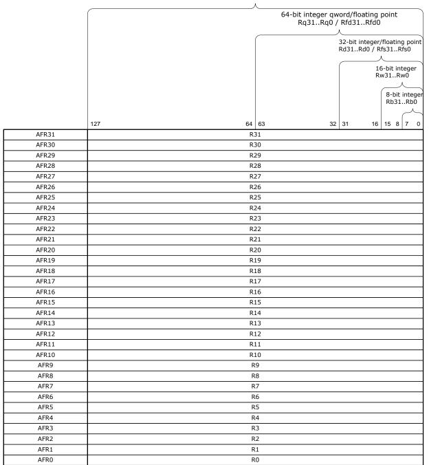
The data of integer formats can be 8-, 16-, 32- and 64-bit. Supports three formats with a floating point - 32, 64 and 128 bits.
