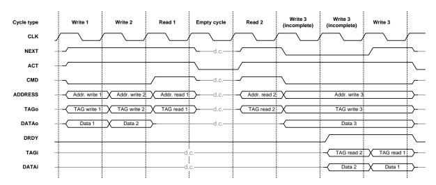
The sequence of data returned by the slave module may not coincide with the order of the read requests generated by the master module. The only way to determine which response to which read transaction has been sent to the master module is the transaction tag. In CoreOne and CoreQuad cores ISI is used everywhere. It connects EU and TMUX, EU and FPU, FPU and stream controller, FPU and TMUX, etc.
