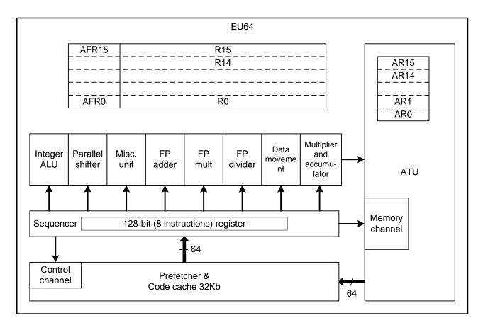
EU X32 contains a 10-channel sequencer also. Unlike from X16 core a X32 core contains divider and multiplier which can process integer operands. Divider and multiplier in core X16 can process only floating point data. Miscellaneous operations unit in the X32 core is able to convert integer to floating point and vice versa. Core X32 prefetcher feeds sequencer by 128-bit bus with throughput up to four instructions per clock. Also prefetcher X32 has 64Kb space of the internal instruction cache.
