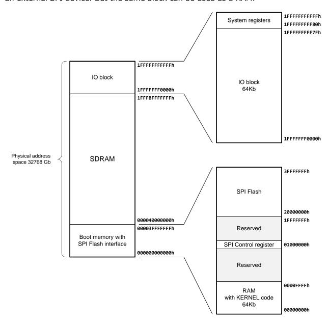
At address 1000000h, the SPI interface control register is located. Writing to it lowest 16-bit word initiates the procedure of transfer a variable number of bytes located from address 0FC00h to the SPI FLASH. The transferred data length is programmed by the contents of the control register.
