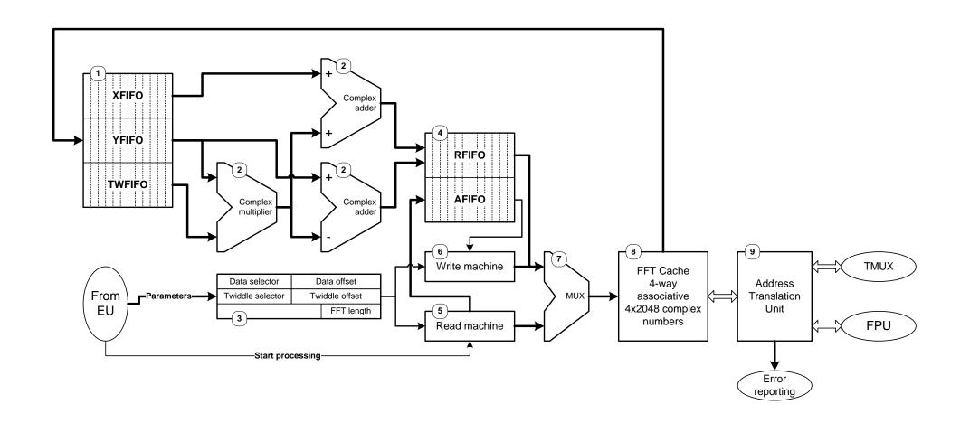
FFT machine consists of the following units.
