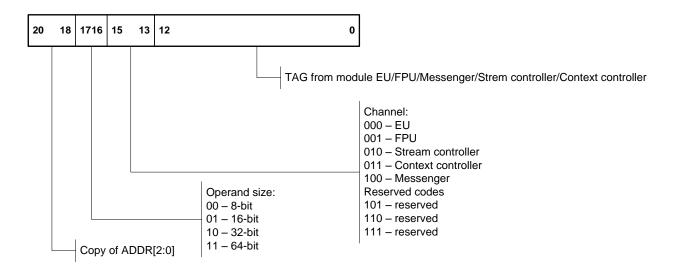
The bit field of the operand size and the copy of the lower three bits of the address are used to determine the SDDAT or IODAT bus lines containing the read data.
