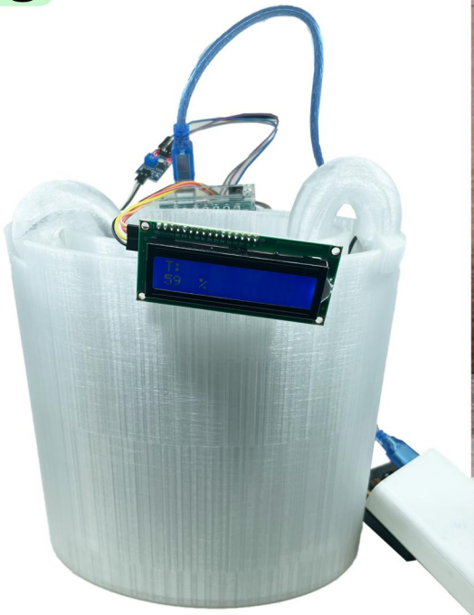
Printed pot integrates soil moisture detection with a water pump.
