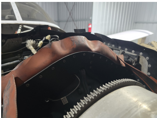
Figure 1 - Wrinkled Front Baffle Seal The front flexible baffle seal is severely wrinkled, folded, and improperly positioned, preventing continuous contact with the upper cowling. The resulting gaps allow cooling air to bypass the cylinders rather than being forced through the cylinder cooling fins.
