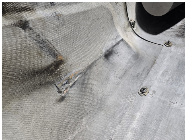
Figure 2 - Evidence of Cooling-Air Bypass Dark airflow and contact marks inside the upper cowling correspond with the baffle-seal location and document cooling air escaping past the baffling. This loss of upper-plenum pressure reduces cylinder-cooling efficiency.
