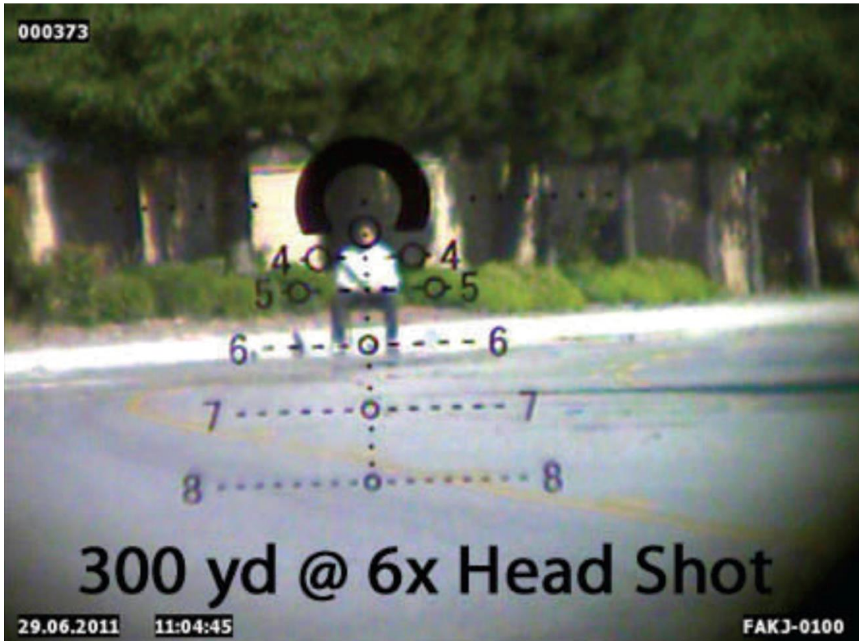
Directly below the horseshoe, to the left and right of the aiming dot on the center line, the ranging circles (labeled No. 4) range a man's head at 400 yards. See photo below.
