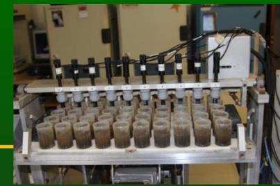
Comparison of soil pH methods shows  $\text{pH (1:1)}_{\text{Salt}}$  is 0.5 pH units lower than  $\text{pH (1:1)}_{\text{H}_2\text{O}}$ .
