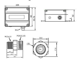
2.N type: M16-8PIN metal connector (RS-485+analog)
