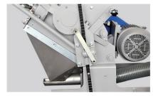
The user friendly design of the E series granulators allows quick and easy access to the cutting chamber for maintenance and cleaning.
