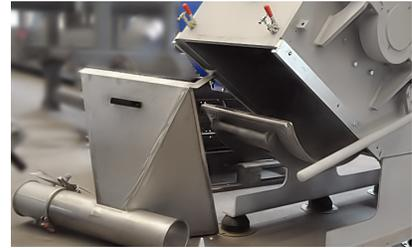
The user friendly design of the E series granulators allows quick and easy access to the cutting chamber for maintenance and cleaning.
