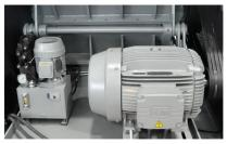
In order to keep the C 70 series as compact as possible, motor and hydraulic opening system are integrated into the sound damp-ening enclosure of the machine.
