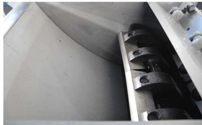
The tangential cutting chamber paired with the aggressive open rotor design ensures reliable ingestion of voluminous parts. The curved cutting chamber backwall reduces the risk of parts getting stuck.
