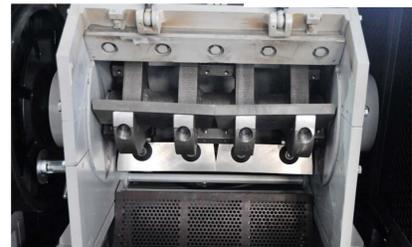
The cutting chamber sits in a soundproofed enclosure to ensure quiet inline operation. The rotor and screen area are easily accessible for cleaning and maintenance without the need for additional tools.
