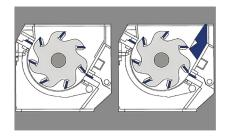
The easily removable deflector wedge acts as a third stator blade and can be used to adjust the aggressiveness of the rotor at the first cutting point.
