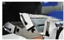
For abrasive applications the H granulators can be equipped with rotors with key parts manufactured from highly wear resistant steel as well as weld on hard facing.
