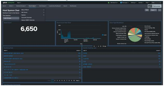
**Intel Analyst Workspace:** This dashboard is designed for an end user that has no prior experience with Splunk or it's query language. It's single panel interface allows the analyst to generate queries, indicators of compromise (IOC) and question future events with a simple point and click of a button.
