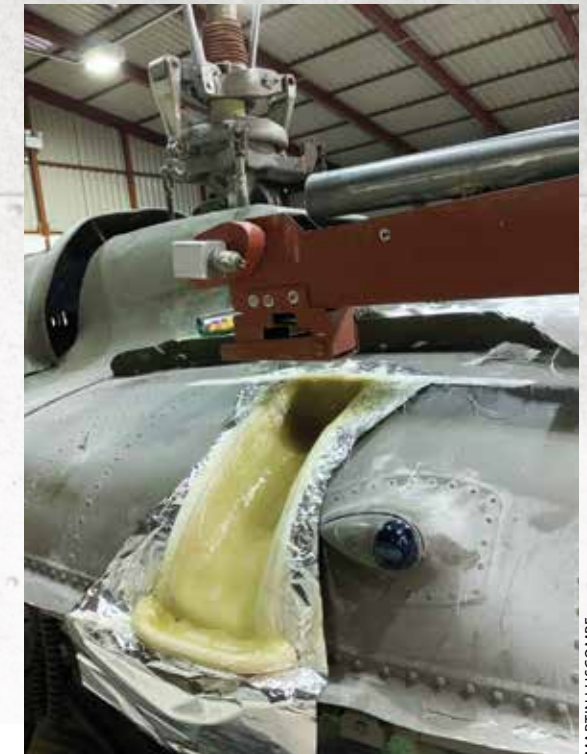
Below: To create the hoist for the Huey, Bird 18 team member Martin Luscombe turned to old photographs to approximate how to build it. He said it was "unnerving" to cut into the helicopter since there was no room for error. He used an old innertube, cut it to shape and glued it in place.
