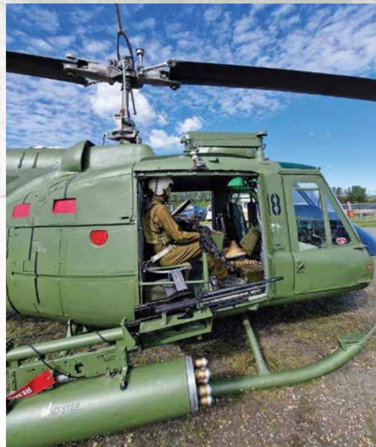
Above: Several of the VMO-6 Marines said the winch looked exactly like the real thing. The two cable guides on the arm are from gym equipment.
