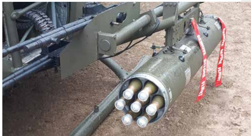
The Bird 18 crew used old photos as their guide and created a TK-2 Weapons platform for the Huey. The M60 machine guns are bespoke replicas created for the project. Several original rocket pods were sourced and then deactivated for use on the helicopter. (Photo courtesy of Stuart Beene)
