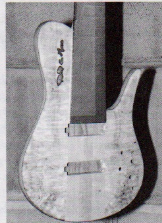
HANGING IN THE SPRAY BOOTH WITH FINGERBOARD TAPED UP READY TO RECEIVE FINISH. NOTICE THE HAND ENGRAVED MOTHER-OF- PEARL SIGNATURE.
