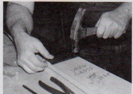
INSTALLING THE FRETS
