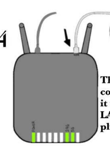
Then check Ethernet cable connect in WAN and follow it to the power supply in LAN and confirm all are plugged in correctly.
