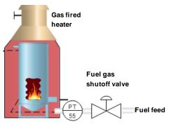
Gas feed to a heater must be carefully monitored to ensure that any reduction in pressure, which could cause a loss of flame, is detected. A 9106 4-20mA repeater IS barrier is used between the pressure transmitter and a safety PLC. When a low pressure event takes place, the safety PLC will send a signal to close the gas shutoff valve, thus preventing a build-up of non combusted fuel in the heater.
