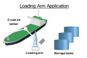
Loading ams are used for the transfer of liquids or compressed gases from tankers and carriers. For safety reasons the loading arm position must be known at all times and must adjust to draft, tide, and positional variations. Numerous limit switches are used to indicate such things as slew angle, apex angle, pulley angle etc. The 9202B switch/pulse IS barrier is used to interface the limit switches with the control system.
