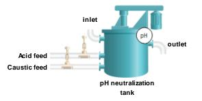
pH control is a process requirement in a wide range of industries, from chemical manufacturing, waste water treatment, life sciencesetc. pH is neutralized by the addition of acid or caustic solutions. pH is measured and solution feed rates are calculated to reach the target pH. A 9107B IS barrier driver is used to supply 4...20 mA from a PLC/controller to an I/P converter which in turn controls the feed valve position.
