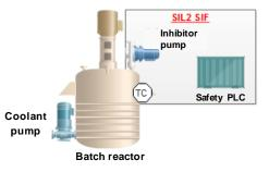
Many chemical reactions are exothermic. Batch reactors often utilize cooling jackets through which cooling water ispumped. If the pump fails, internal temperature rises causing a runaway reaction and possible explosion. To prevent this, a 9113 temperature IS barrier can be used aspart of an over-temperature SIL2 safety function. The safety system will inject a reaction inhibitor when over-temperature is detected.
