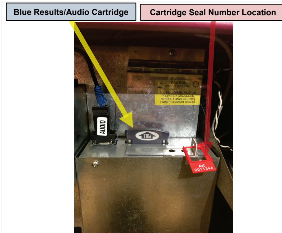
Figure 50: Results/Audio Cartridge Port Location and Removal (Part 1)
