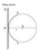
A circle is drawn from the centre (O) such that it just touches the plane mirror at point O'. According to Huygens' Principle, XY is the wavefront of incident light.
