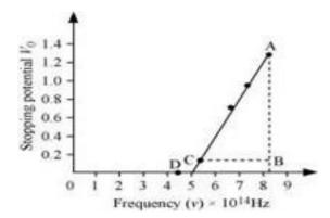
It can be observed that the obtained curve is a straight line. It intersects the v-axis at  $5\times 10^{14}$  Hz, which is the threshold frequency  $\left(v_0\right)$  of the material. Point D corresponds to a frequency less than the threshold frequency. Hence, there is no photoelectric emission for the  $\lambda_5$  line, and therefore, no stopping voltage is required to stop the current.
