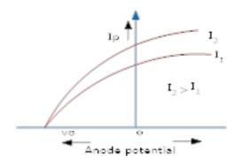
(iii) Photoelectric current is directly proportional to the intensity of incident radiations, provided the given frequency is greater than the threshold frequency.
