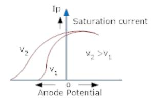
(ii) Stopping potential does not depend on the intensity of incident radiations.
