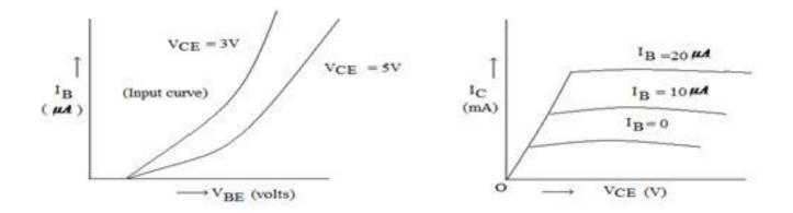
output characteristics is the variation of the collector current  $(I_{\mathcal{C}})$  with collector emitter voltage  $(V_{\mathit{CE}})$  at constant base current  $(I_{\mathcal{B}})$  is called output characteristics.
