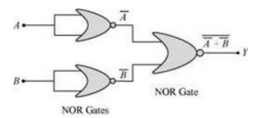
$\overline{A}$  and  $\overline{B}$  are the inputs for the last NOR gate. Hence, the output for the circuit can be written
