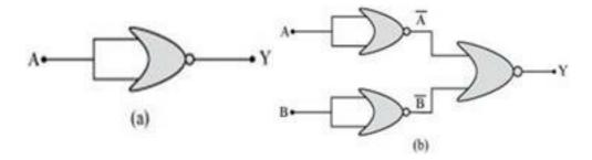
**Ans.(a)** A acts as the two inputs of the NOR gate and Y is the output, as shown in the following figure. Hence, the output of the circuit is  $\overline{A+A}$ .
