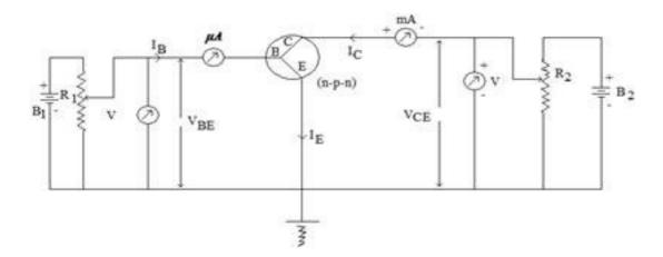
Input characteristic curve is the variation of base current  $I_{\it E}$  (Input) with base – emitter voltage (VEB) at constant collector emitter voltage ( $V_{\it CE}$ ).
