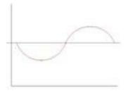
Relation – output waveform has  $180^{\circ}$  phase reversal as compared to input and also the output is being amplified.
