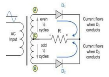
Suppose for positive half of a.c. input diode  $D_1$  is forward biased and  $D_2$  is reverse biased, then the current will flow across  $D_1$  where as for negative half of a.c. input diode  $D_2$  is forward biased and the current flows across  $D_2$ . Thus for both the halves output is obtained and current flows in the same direction across load resistance  $R_2$  and thus a.c. is converted into d.c.
