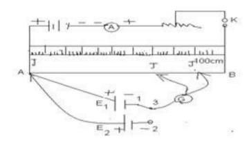
(Condition – close the switch and 3 such that  $\,E_{\rm l}\,{\rm comes}$  in the circuit)
