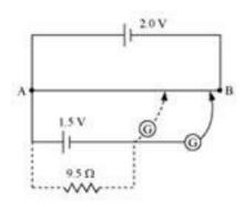
An external resistance (R) is connected to the circuit with  $R = 9.5\Omega$
