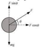
The vertical component of this applied force acts upward. This reduces the effective weight of the mower.
