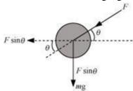
In this case, the vertical component of the applied force acts in the direction of the weight of the mower. This increases the effective weight of the mower.
