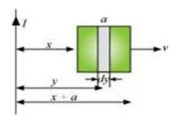
**(a)** Take a small element *dy* in the loop at a distance *y* from the long straight wire (as shown in the given figure).
