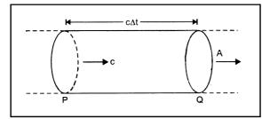
The energy of electromagnetic wave (U) crossing the area of cross-section at P normally in time  $\Delta$  t is the energy of wave contained in a cylinder of length c  $\Delta$  t and area of cross-section A. It is given by  $U = u_{av}$  (c  $\Delta$  t) A
