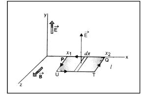
Consider a rectangular path PUTQ in the X–Z plane as shown in figure. The line integral of  $\vec{B}$  over the closed path PUTQ, we have
