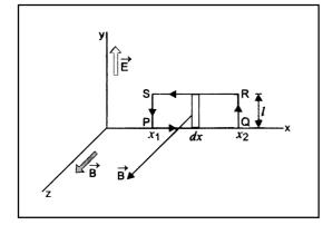
The line integral of  $\vec{E}$  over the closed path PQRS will be
