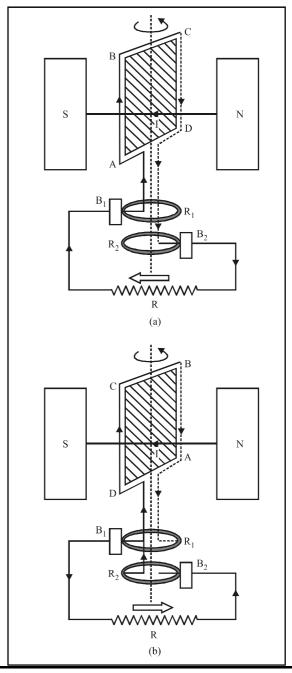
After half the rotation of the coil, AB is at the back and CD is at the front, figure. Therefore, on rotating further, AB moves outwards and CD moves outwards and CD moves inwards. The current induced in AB is from B to A and in CD, it is from D to C. Through external circuit, current flows from  $B_1$  to  $B_2$ ; figure (b). This is repeated. Induced current in the external circuit changes direction after every half rotation of the coil. Hence the current induced is alternating in nature.
