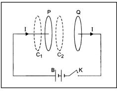
Due to battery B, let the conduction current I be flowing through the lead wires at any instant, but there is no conduction current across the capacitor gap, as no charge is transported across this gap.
