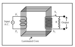
For an ideal transformer, we assume that the resistances of the primary and secondary windings are negligible. Further, the energy losses due to magnetic hysterisis in the iron core is also negligible. Well designed high capacity transformers may have energy losses as low as 1%.
