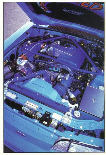
1-5/8 inch Motorsport headers. A high-volume fuel pump supplies ample juice to the high-output engine while a heavy-duty four-core radiator keeps the internals at a comfortable operating temperature. Bringing up the rear is a Borla stainless steel exhaust system accented with Hedman exhaust tips and custom valence trim.
