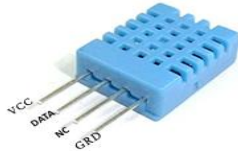
Figure 8: Temperature and Humidity Sensor
