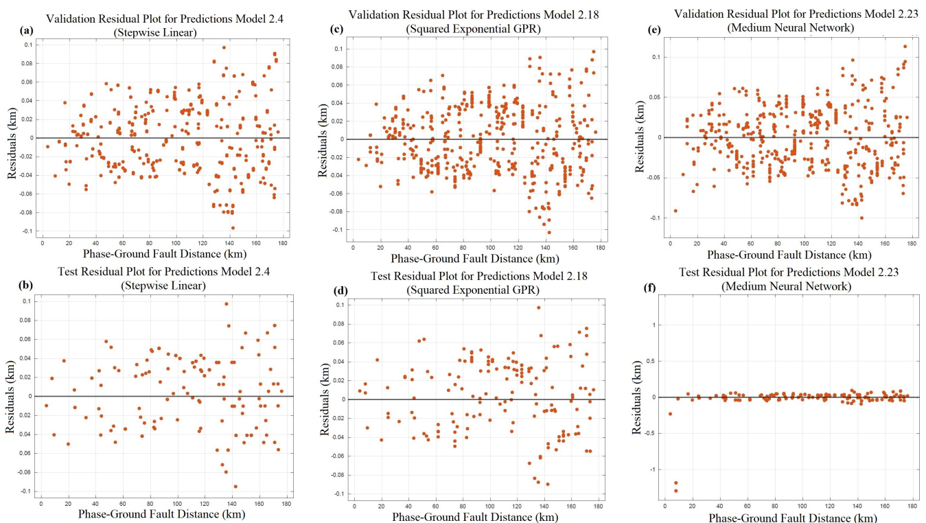
Figure 10. Residual difference plots at various km points for phase-to-ground failures. (a) Linear regression for validation. (b) Linear regression for testing. (c) Gaussian process for validation. (d) Gaussian process for testing. (e) NN for validation. (f) NN for testing.
