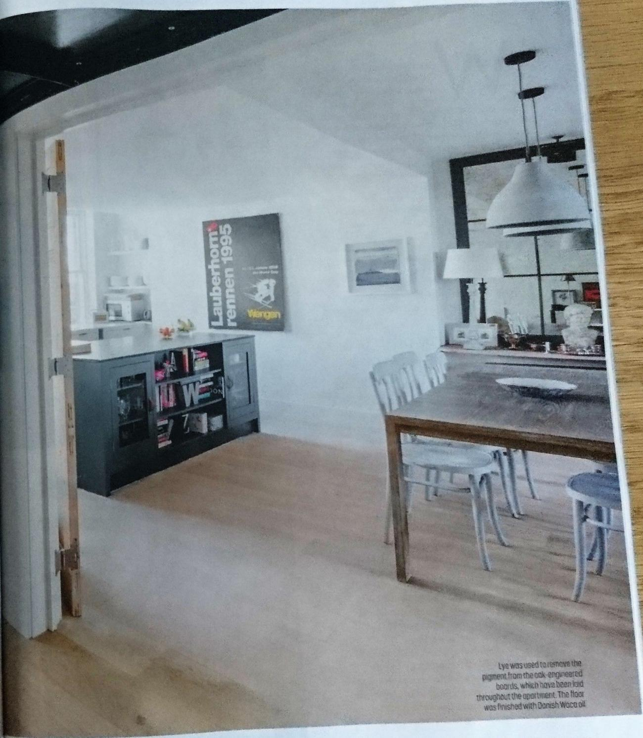
Lye was used to remove the pigment from the oak-engineered boards, which have been laid throughout the apartment. The floor was finished with Danish Waco oil.
