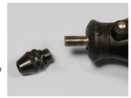
A simple and inexpensive (\$12) adjustable chuck solves all of this. It's available in most large local hardware stores or modelmaking outlets. Tightening the chuck is done easily by hand to any size shaft. No key is required.
