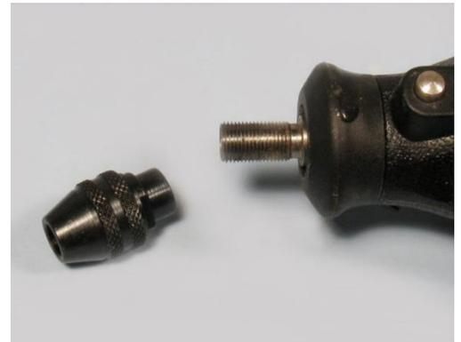
The basic motor tool as sold typically comes with a collet chuck. This means you have to use a wrench to change every tool bit, you have to switch collets to use different shaft sizes (3/32 or 1/8 inch bits), and you can't use ordinary drills at all - only the special ones that have a 3/32 shaft.
