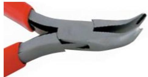
The easiest way to create a slot on the pusher is with a file, and the quickest way to create a slot on one jaw of your pliers is with a separating disc. Then do a rough polish on the slot with a medium grit, knife-edge silicone wheel.
