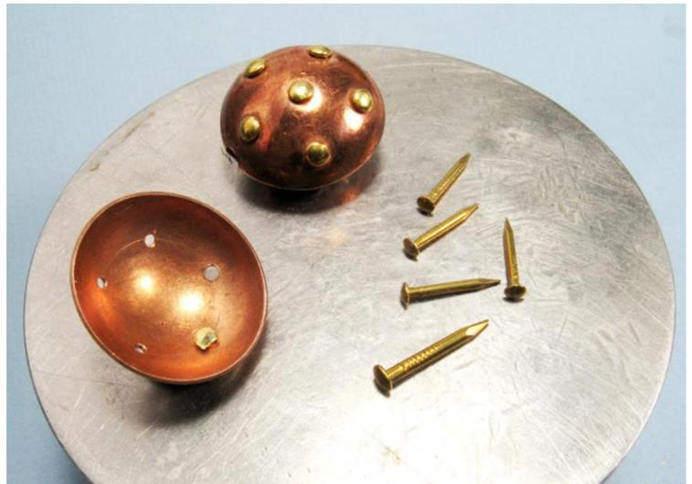
For best results, select a drill that gives you a hole with a close fit to the rivet. Trim the rivet to a leave a little less than one diameter sticking out the back side. Place the head on a scrap of hard plastic on the anvil so as to not flatten the head. I prefer a ball peen hammer (with a small 3/8-inch ball) for setting the rivet.
