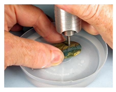
One of the things my students often ask to do is drill a hole through a piece of gemstone. The usual thought is to get a diamond drill, but I've been disappointed with them. I think the reason is that the tip of the drill is just pivoting in the hole and fails to cut well. When it looks like the drill isn't cutting, the tendency is to push with more force. The drill gets hot, and the diamond grit falls off.
