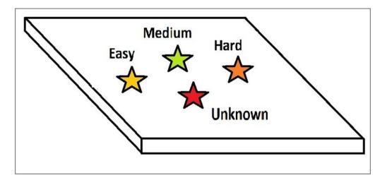
There are plenty of ways to mark your sheet or wire solders, but suppose you forgot to mark them and have a couple that you can't identify. The answer is to compare the melting temperature of the unknowns with that of a known solder.
