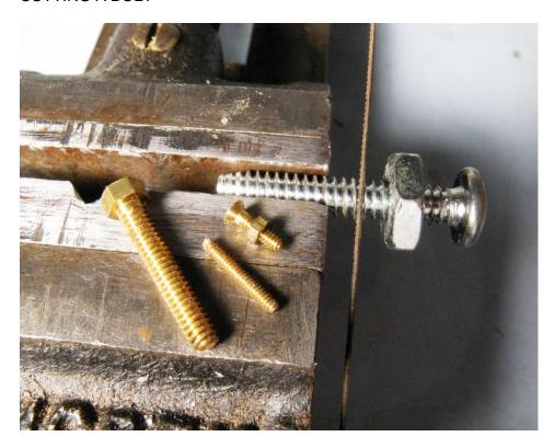
Whenever you have to cut a threaded bolt shorter, it's often difficult to get the nut to thread back onto it. And the smaller the bolt, the more difficult it is to restore any distorted threads. The problem is easily solved with the use of a nut. Here's how I do it.
